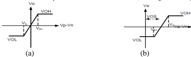
Fig.3: (a) Transfer curve of a comparator with infinite gain (b) Transfer curve of a comparator including input - offset voltage
