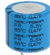
Fig: 7 A Typical Ultra-capacitor
