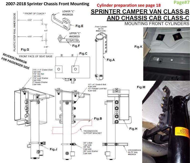
The front cylinder setup is the same on a Sprinter Chassis Cab Class-C and a Sprinter Camper Van Class-B. First, locate area under vehicle front cab in front of the driver's seat on the outside face of the frame. See (Fig.B and Fig.M) above showing the transmission support bracket attached to the frame, our cylinder's Lower "L" Bracket (Fig.E) will slide between that support bracket and the bottom face of the frame (Fig.C).
