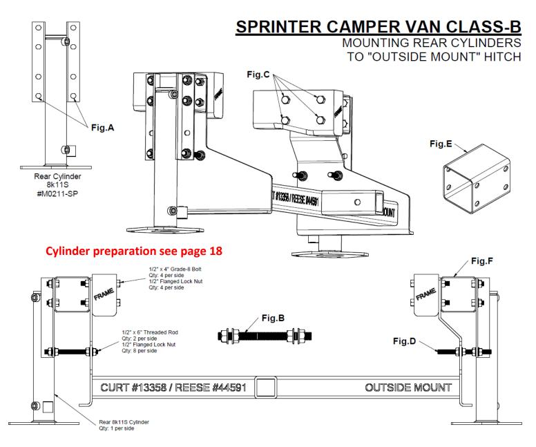
Typical Sprinter Van's have two basic hitch options: 1. "Inside Mount" which refers to the mounting plates bolting in-between the frame rails on the inside surface. 2. "Outside Mount" which refers to the mounting plates mounting on the outside surface of the frame rails.
