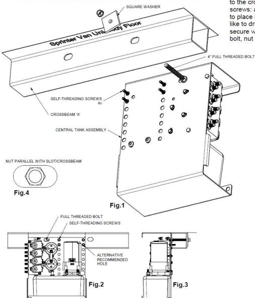
Locate the crossbeam shown to the left. The tank assembly can be mounted on either the front or rear face of the crossbeam.
