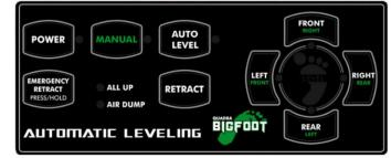
Make sure all four cylinders are retracted, if they are move to step 2. If not, turn panel ON, let diagnostic lights flash until they stop (within 30 seconds). Press RETRACT button, when all up light comes, move on.
