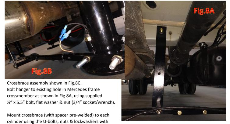
under limit switch barrel and between limit switch pin and cylinder housing. Crossbrace should be just above the footpad, and mounted to rear side of cylinder, Fig.8B.
