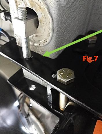
BOTH BRACKET LIFTING SURFACES MUST BE TIGHT TO BOTTOM OF FRAME, HOLE CATCHER WILL BE ON OPPOSITE SIDES FROM DRIVER TO PASSENGER CYLINDER.
