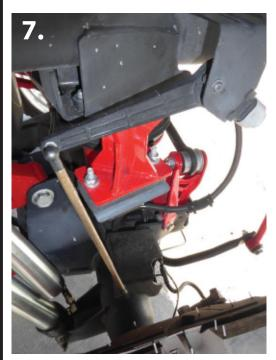
Make sure before you set the truck on the ground. That the top of the factory air spring/bag, locks in to the original bag mount on the frame, and cannot fall out. Also check, to make sure all your lines are clear of any moving parts that could cause any rubbing or failure. Make sure nothing is rubbing against any of the air lines or the factory air bags.
