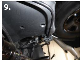
7. Underneath the factory track bar mount, there is a small hole that needs to be drilled out to 1/2". (pic 8-9)
