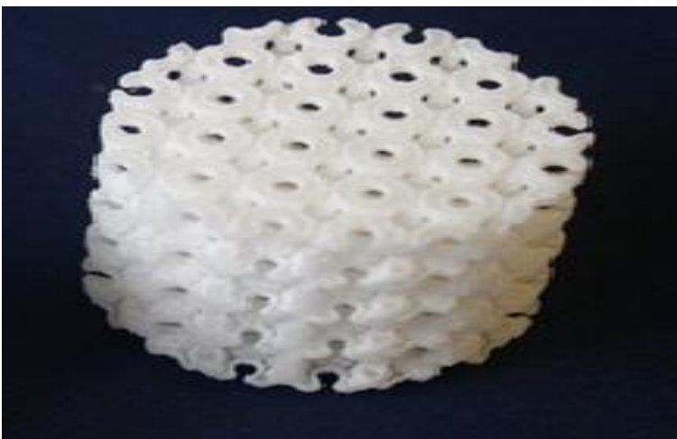
Figure 2: showing 3-D synthetic polycaprolactone scaffold. [6]
