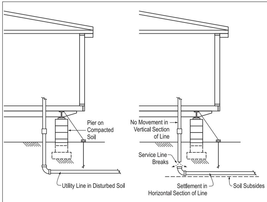
Figure 2-8. Utility line damage in unstable soils.
