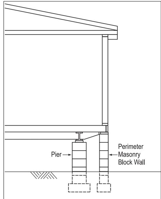
Figure 2-7. Perimeter wall foundation under a manufactured home.
