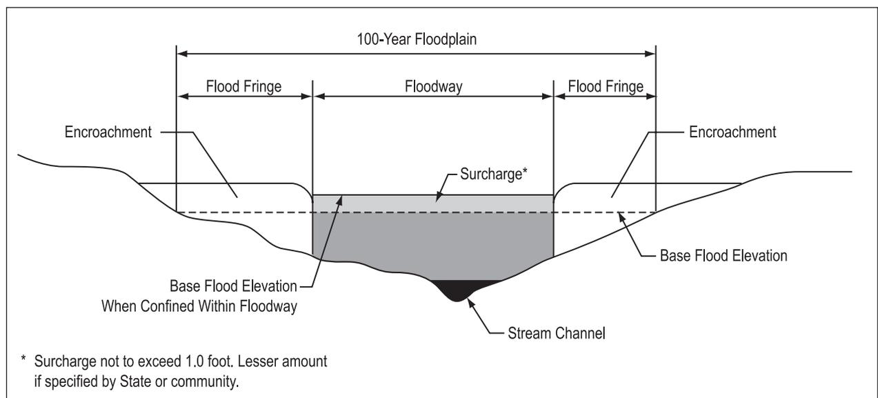
Figure 4-2. Floodplain/floodway schematic.
