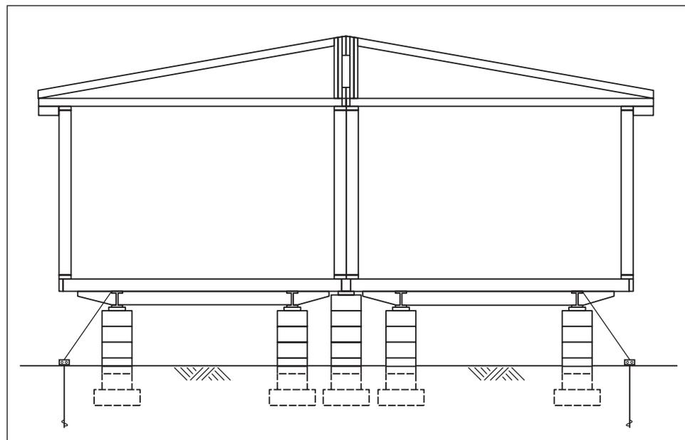
The advantages of this foundation system are that it adapts easily to the site conditions, does not require much dimensional precision, is installed very quickly, and is economical to install.
