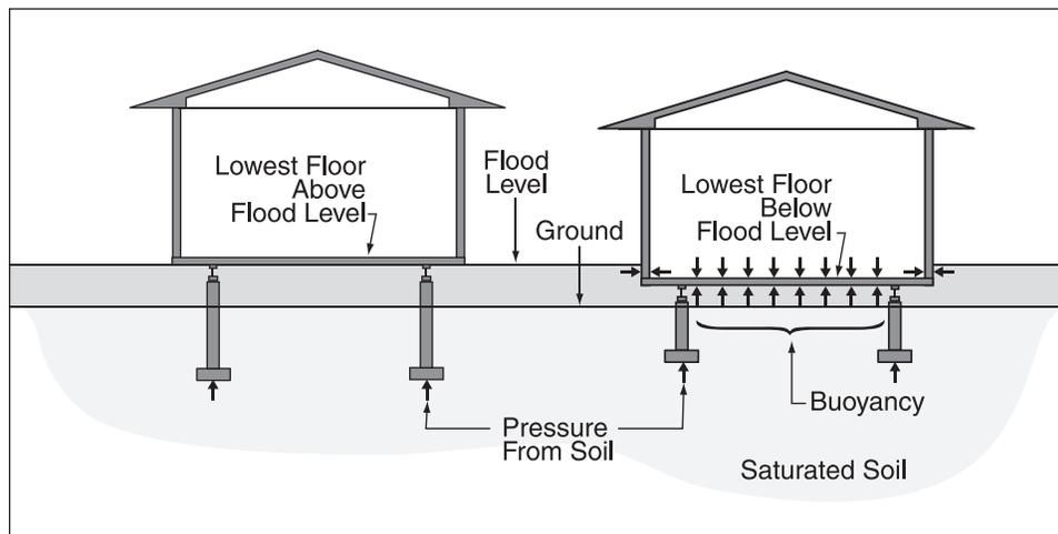
**Figure 5-5. Buoyancy forces acting on a structure.**
