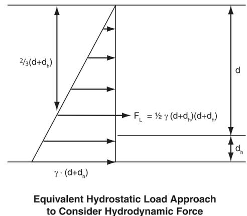
An alternative approach to consider the dynamic effects of moving water is to use an equivalent hydrostatic load approach. When water velocities are less than 10 fps, ASCE 7 permits adding an equivalent surcharge water depth to the design flood elevation to simulate the hydrodynamic load.
