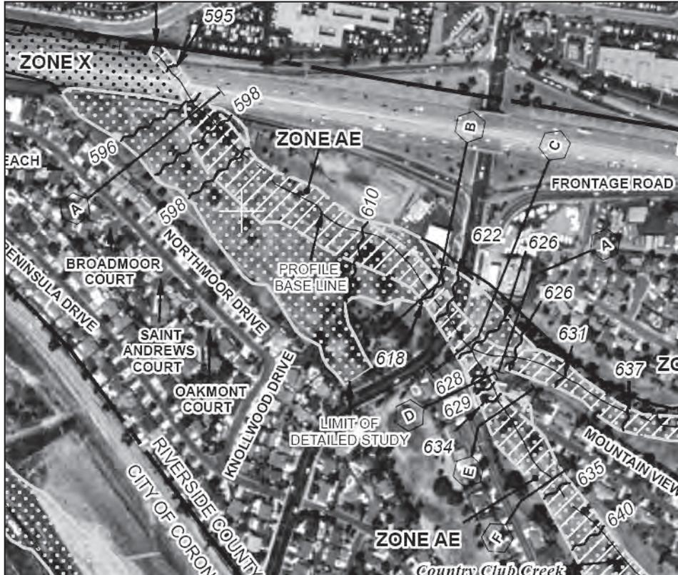
Figure 3-5. DFIRM showing the floodway (cross-hatched area in Zone AE).
