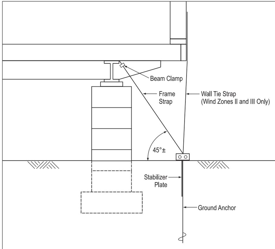
Figure 7-4. Typical ground anchor installation.
