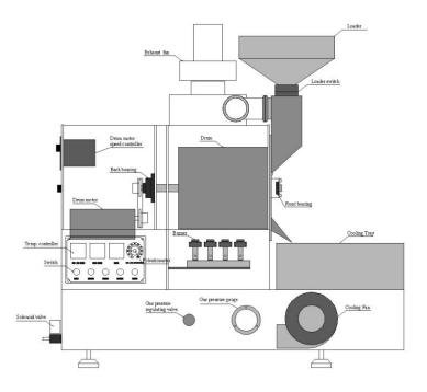
THE BC-5 MD IS A HEAVY DUTY ROASTER BUILT WITH A CARBON STEEL BODY WITH APPROVED POWDER COAT HIGH TEMPERATURE BODY IN BLACK. THE HOUSINGS COME IN A CHOICE OF 4 COLORS (Gold, Rose Gold, Black Titanium & Stainless) In two type finishes (MIRROR or MATTE) TWO EXHAUST PIPES COMES OFF THE BC-3 AT 3" AS SHOWN BELOW AND CAN BEEXHAUSTED OUT OF BUILDING SEPARATELY OR CONNECTED WITH A BLAST OR BACKDRAFT DAMPE
