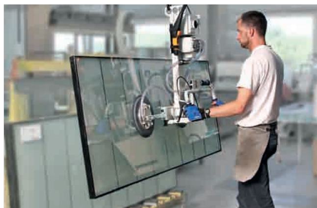
Vacuum lifting device VacuMaster Window for vertical handling of glass elements
