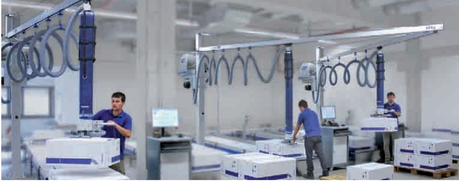
Vacuum tube lifter JumboErgo for lifting cardboard boxes
