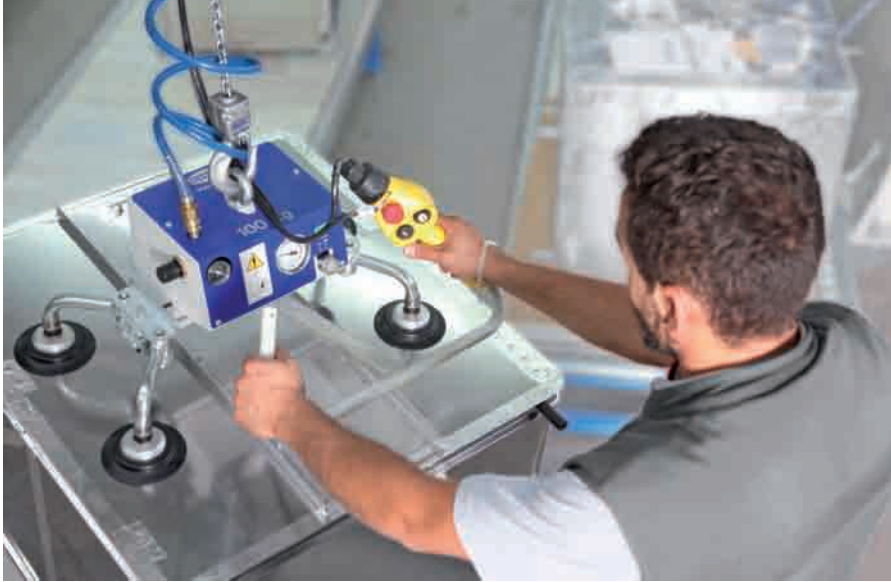
VacuMaster Light for handling metal housings
