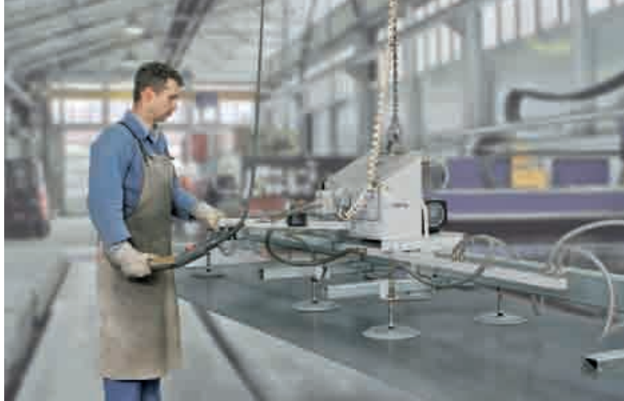
VacuMaster Vario in process of loading and unloading a laser cutting machine
