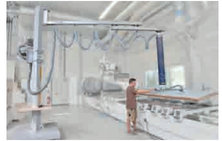
Telescopic jib for confined working areas
