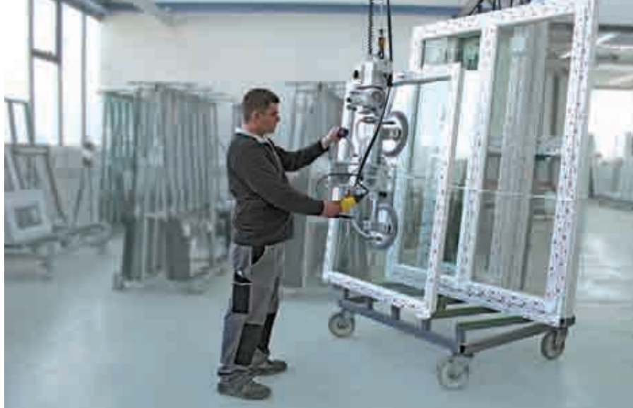
VacuMaster Window for rotating and palletizing windows
