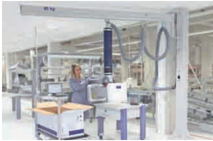
Flat jib for particularly low ceilings
