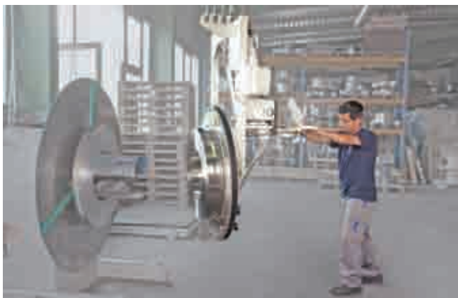
Vacuum lifting device VacuMaster Coil with 90° swivel angle for handling coils
