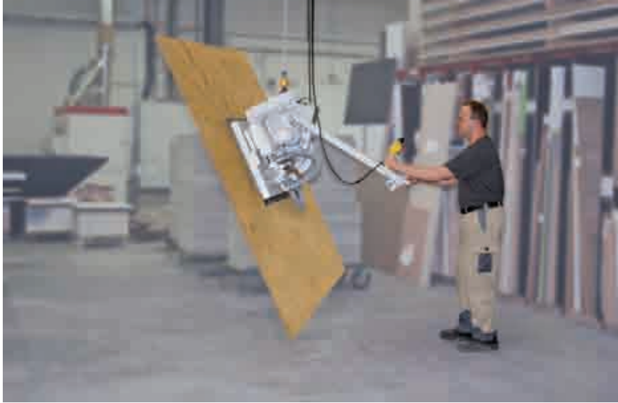
VacuMaster Multi for swiveling wooden boards by 90°
