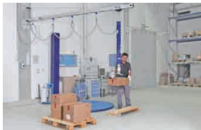
Wall-mounted jib crane WK with vacuum tube lifter Jumbo
