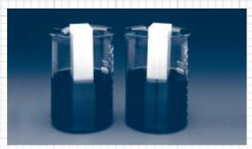
A simple dye penetrant test highlights the significance of porosity in some acetal shapes.
