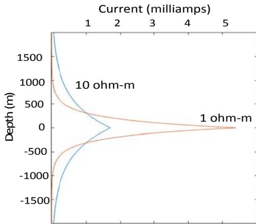
**Figure 1.** Leakage current from pole source along an infinite steel pipe of conductivity  $5.5 \times 10^6$  and thickness 1 cm in a homogeneous medium
