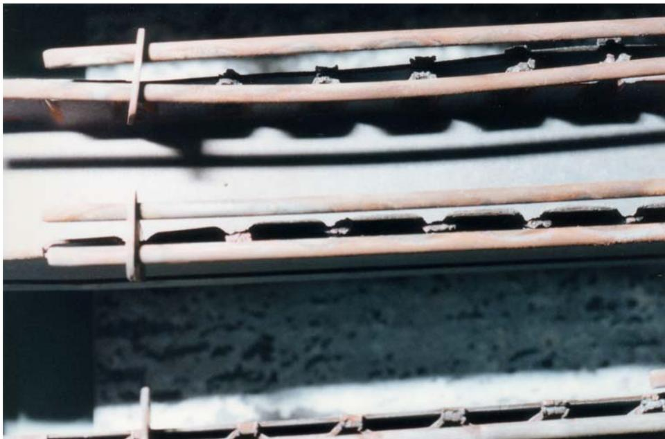
**Photo Four: Damaged NOX rod equipped burner assembly.**
