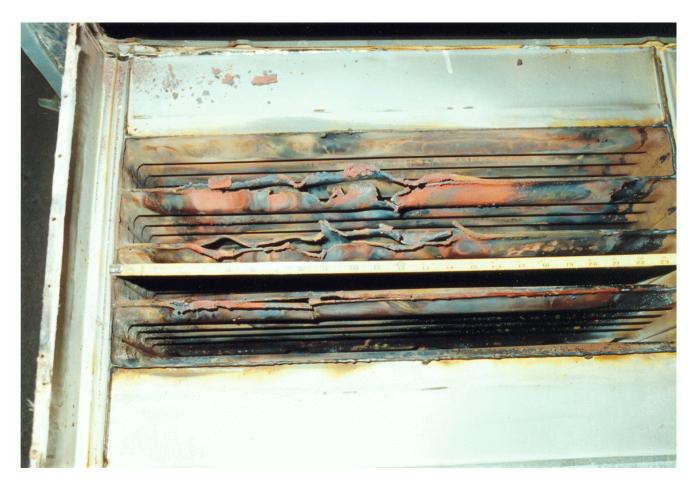
Photo Seven: Major failure of heat exchanger.
