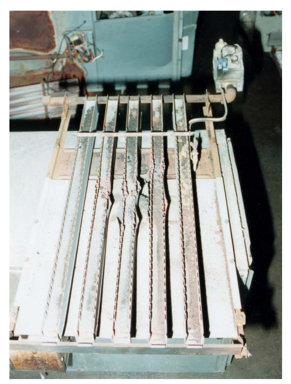
Photo Five: Damaged burner assembly <u>not</u> equipped with NOX rods.
