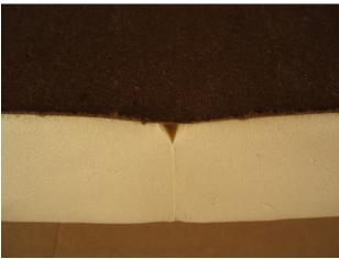
Knit line and V-groove close-up (after conditioning)
