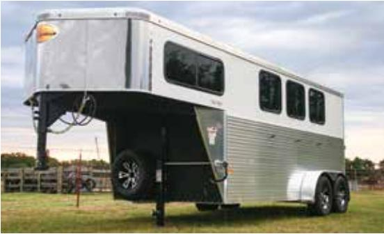
Known for its trailers' value and innovation, Sundowner has made several safety features standard in all of its models this year, including nitrogen-filled tires and rubber torsion axles.
