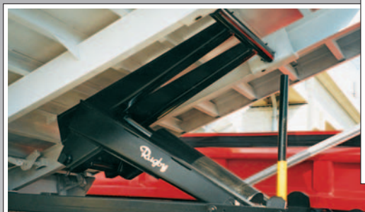
Dump Body Package Includes LR Series Hoist
