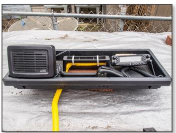
Figure 22. The top tray holding the radio head and speaker may be removed from the box for convenience.
