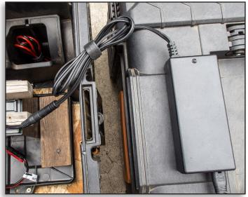
Figure 25. Bioenno charger connected to the battery.
