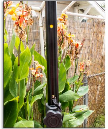
Figure 20. The center tube of the tripod may be extended to give the antenna more height.
