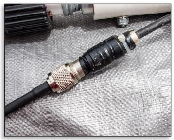
Figure 18. Coaxial cable connected to antenna pigtail.
