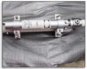
Figure 16. Antenna base inserted into mounting brackets.
