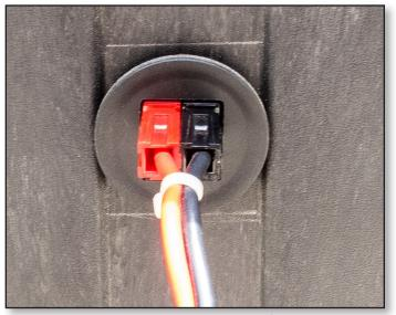
Figure 8. Power connection on the back of the radio box.
