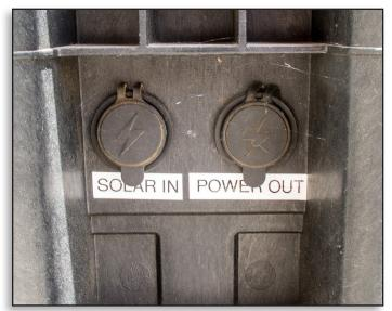
Figure 4. Battery box rear connections.
