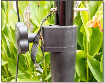
Figure 21. The securing knob on the tripod showing the pin inserted to extend the mast height.
