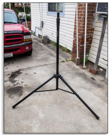
Figure 11. Antenna mast support tripod.
