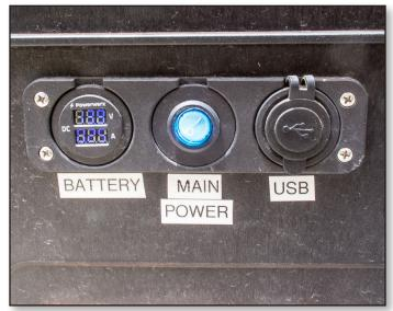
Figure 24. Main power switch on the battery box.
