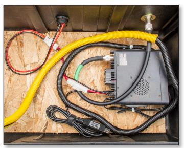
Figure 5. Radio box showing body of the FT-8800R.
