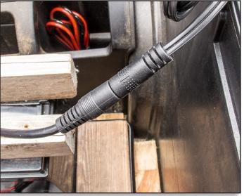
Figure 26. Close up of the Bioenno charger connected to the battery.
