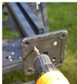
4) Secure with the 5 included screws.
