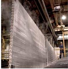
Heated alkaline cleaning process to remove contaminants
