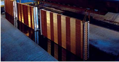
Factory-applied ElectroFin E-coat solution
