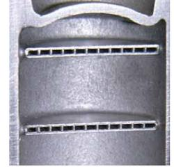
Manifold cross-section for micro-channel heat exchanger
