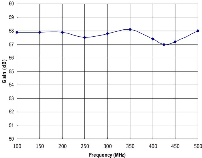
Figure 1: RFM100-500-350-HSD Typical Gain @  $P_{out} = 350W$ .
