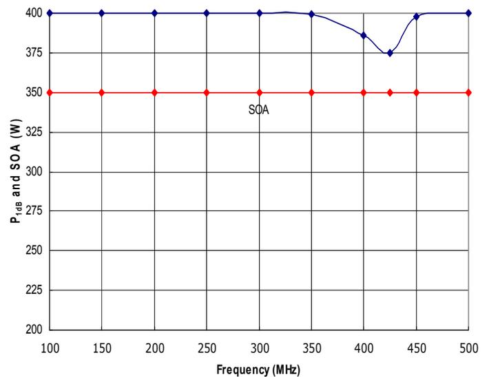
Figure 4: RFM100-500-350-HSD Typical  $P_{1dB}$  and Safe Operating Area (SOA). The amplifier is capable of delivering more power than it is safe to generate. **Do not exceed the SOA shown above without first contacting RFMPT to discuss your application.**
