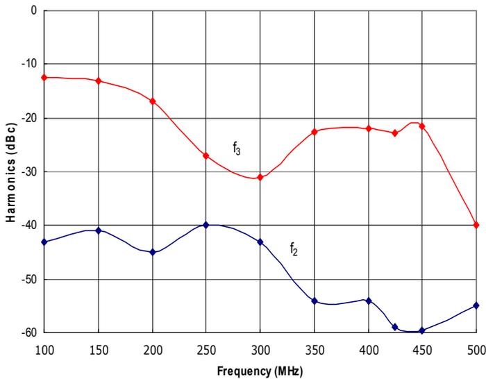
Figure 3: RFM100-500-350-HSD Typical  $f_2$  and  $f_3$  @  $P_{out} = 350W$ .
