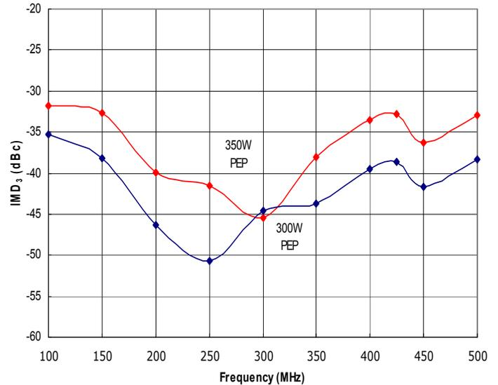
Figure 2: RFM100-500-350-HSD Typical  $IMD_3$  @ 350W and 300W PEP,  $\Delta f = 100kHz$ .
