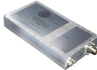
The RFM100-500-350-HSD is a high gain, high power Class A/AB amplifier module designed for military and commercial communications systems. It features fast output disable with  $\leq 1\mu\text{sec}$  response time, and includes numerous control and monitoring functions. It exhibits excellent gain flatness and linearity, and is offered in a compact housing with a nickel plated copper base for best possible thermal performance.
