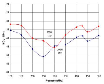
Figure 2: RFM100-500-350-HSD Typical IMD<sub>3</sub> @ 350W and 300W PEP, Δf = 100kHz.
