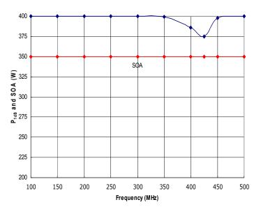
Figure 4: RFM100-500-350-HSD Typical  $P_{1dB}$  and Safe Operating Area (SOA). The amplifier is capable of delivering more power than it is safe to generate. Do not exceed the SOA shown above without first contacting RFMPT to discuss your application.
