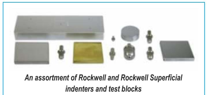
*An assortment of Rockwell and Rockwell Superficial indenters and test blocks*
