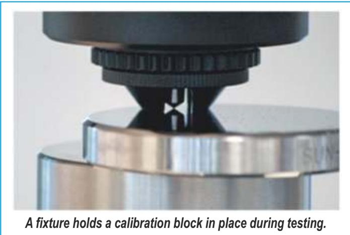
*A fixture holds a calibration block in place during testing.*
