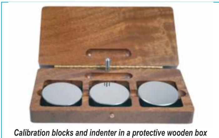
*Calibration blocks and indenter in a protective wooden box*
