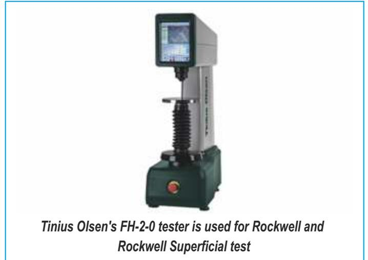
*Tinus Olsen's FH-2-0 tester is used for Rockwell and Rockwell Superficial test*
