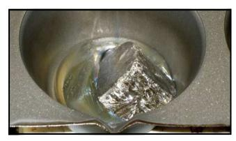
Melting bismuth in a cupcake pan. The pan has been cut apart and a pour spout has been bent into one side.
