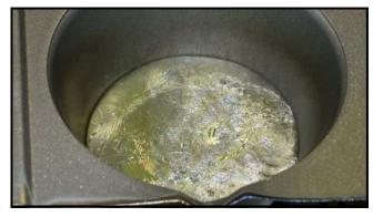
Melted bismuth showing the yellowish slag floating in the top of the liquid. The slag can be removed with a stainless steel kitchen fork.
