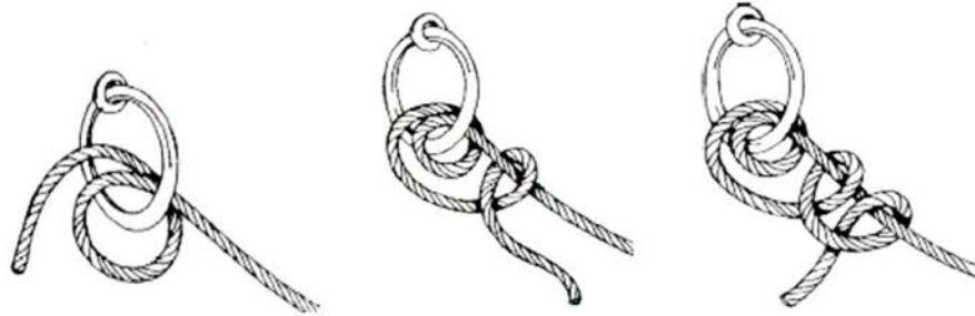
CFC D 105 Seamanship Rigging and Procedures Manual Figure 10-1-6 Round Turn and Two Half Hitches
