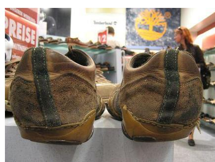
Lateral (excessive or uneven) wear pattern
