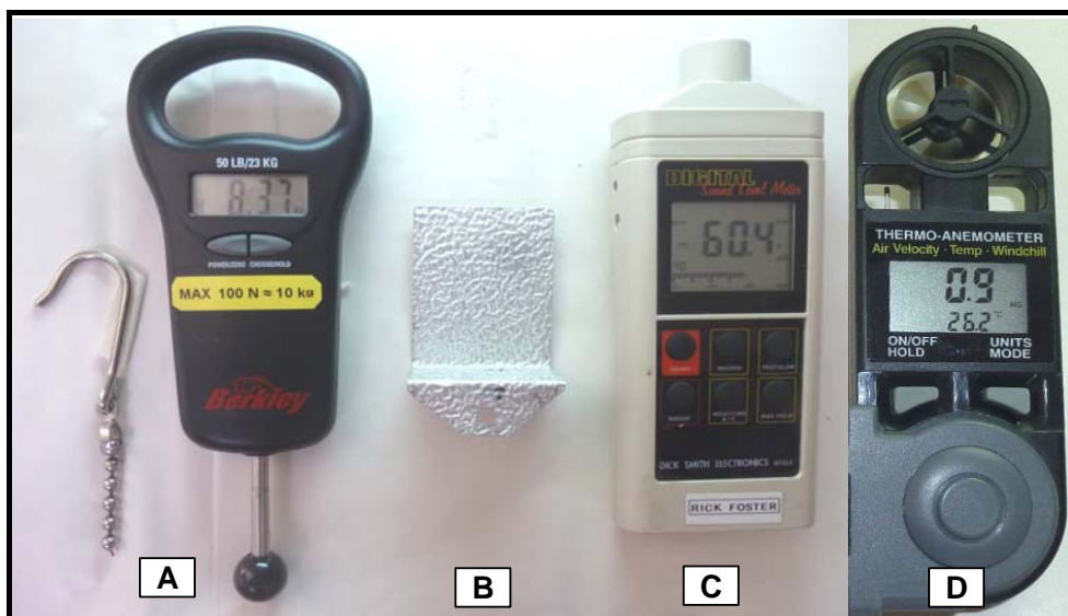
Figure 1 – Stair Pressurisation Instruments
