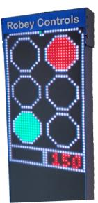
The controller's status is shown at the top of the PLT along with any potential error code that may exist for the carousel.
