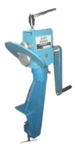
The Easy Edger is used to form the curved and radius 90° Male flange seam edges of sheet metal. The handle at the top of the unit is used to set the depth of the forming roll. Rotating the large handle to the side turns the forming rolls.
