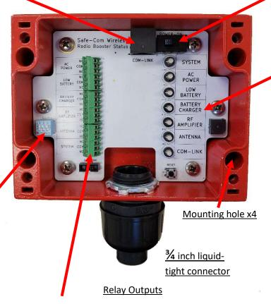
Form C Relays are provided for connection to a fire panel. For each of the 6 NFPA alarms a relay output is provided. Select the two ports depending on the fire panels input requirement: either normally open or normally closed along with the common.
