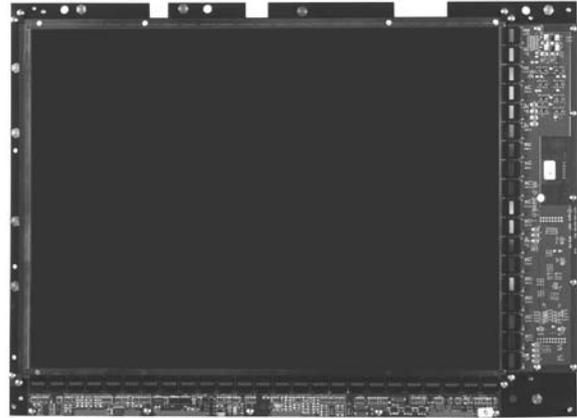
Fig. 1: A 30x40 cm<sup>2</sup> imager module with gate and data boards TAB bonded to the glass and mounted on an aluminum frame.
