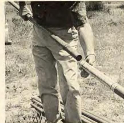
As he lays the poles on the ground, he slips them together. He made sleeves of aluminum and the poles from stair railing.
