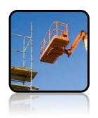
Involved in falls from the platform include static boom (1b) type machines (30.8 percent of incidents), mobile vertical (3a) types (28.8 percent) and mobile booms (3b) (22.8 percent).
