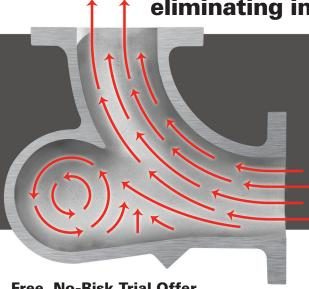
Unlike conventional "impact" elbows and "plugged-tee" elbows that rely on material impact to change direction, HammerTek's Smart Elbow® design employs a spherical chamber that protrudes partially beyond the desired 90° or 45° pathway, causing a ball of material suspended in air to rotate. Since the ball of material rotates in the same direction as the airstream that powers it, incoming material is cushioned by the ball's rotation, and is gently deflected around the bend.
