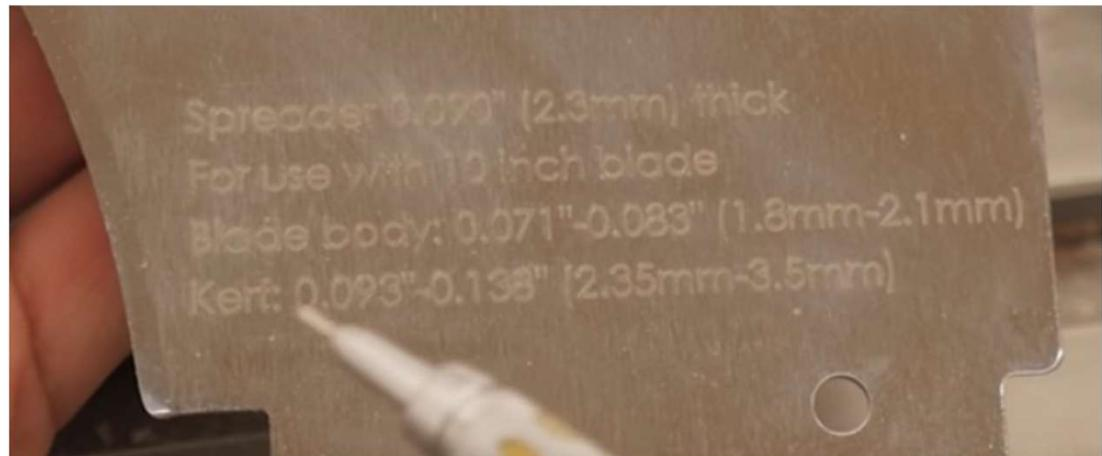
**Coordinate the riving knife / splitter with the blade body width and/or blade kerf.**
