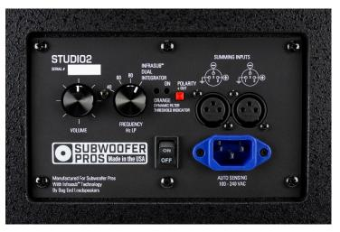
The SUBWOOFER PROS Studio Sub2-12C is a "universal" sub used for bass extension of any studio monitor. It is sealed and self-powered, offering bass extension to 16Hz. It has a compact cabinet using a 12" high excursion sub driver with an easy to use control set. It has built in Left/Right XLR summing inputs and a low pass filter at 4 different frequencies of 95Hz, 80Hz, 60Hz, and 40Hz. The different low pass frequencies make it adaptable to various size "main" speakers.
