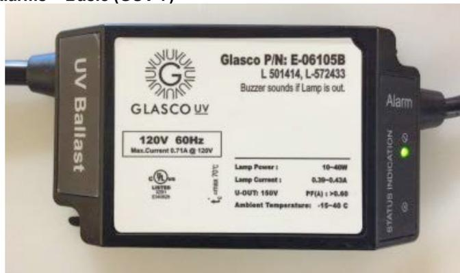
The unit will have come with an audible and visual lamp status alarm. In the event of a lamp out, the audible alarm will sound. The green light aka LED indicates lamp is on, the LED will go off when the lamp goes off and the red LED will illuminate. If this is the case, have your water professional check to see if the lamp needs to be replaced. When alarming, the water may not be safe to drink.
