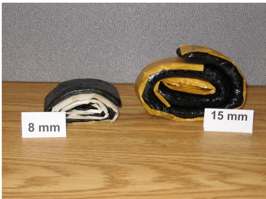
The asphalt tape (Photo 7) is applied to the cold joint in advance of the paver. At the time of writing this, the use of these tapes are still at the trial stage. In trials, there were ongoing issues with workmanship relating to the placement of the tape that may have influenced the success of the trials.
