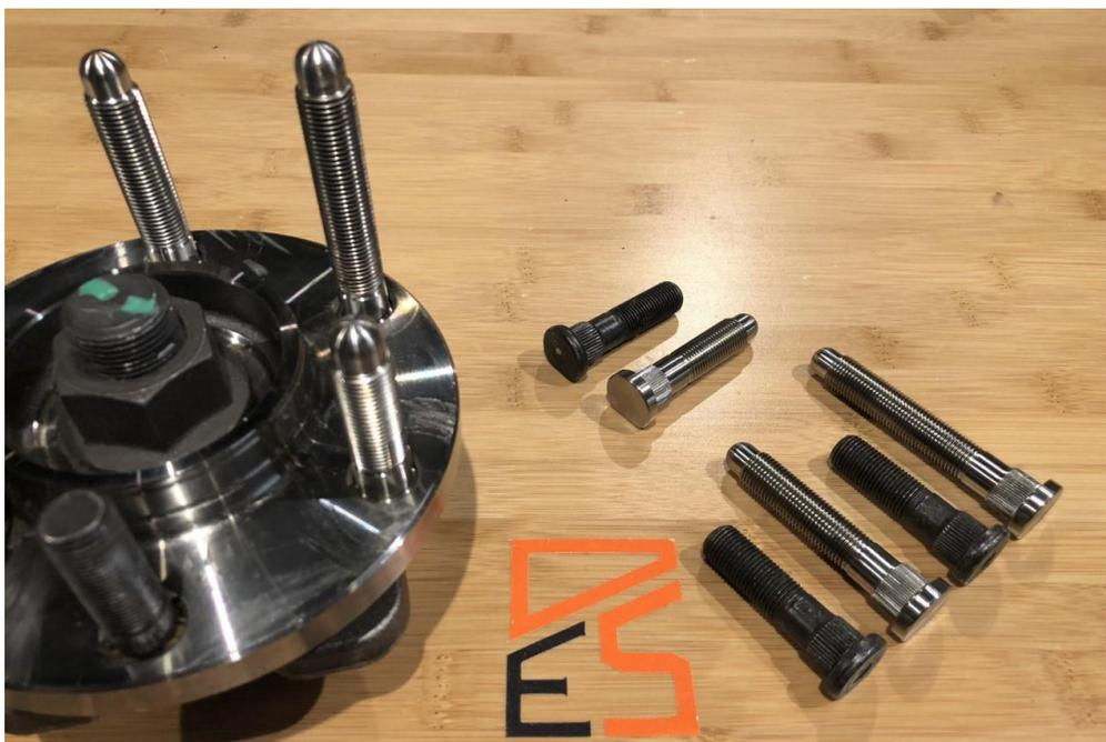
***Studs of each length installed on a Viper hub aside OEM studs for comparison***
