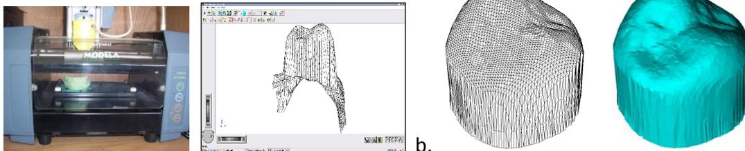
Figure 1: a. 3D Scanner & screen shot of scanned crown, and b. final crown model
