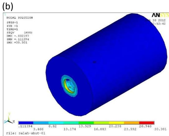
**Figure 4:** Von Mises stress of spongy bone under zirconium crown, and Glass ionomer cement layer with (a) equal and (b) non equal distributed vertical loading of 300N. (R41, 42)
