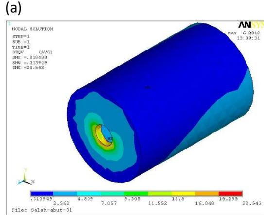
**Figure 3:** (a) In-Ceram and (b) zirconium crowns Von Mises stress distributions when loaded by 200N at Palatal Cusp Tip & 100N at Central Fossa. (R18, 42)
