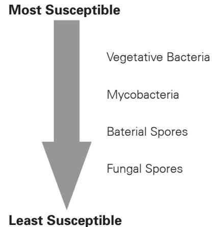
In addition to inactivating airborne microorganisms, UVGI directed at environmental surfaces can damage culturable microorganisms present or growing on the surface. Lower-intensity UVGI is effective for surface inactivation because irradiation is applied continuously. UVGI from lamps in AHU plenums has been used successfully to inactivate microorganisms present on airstream surfaces such as on cooling coils and drain pans (Menzies et al. 1999, 2003).
