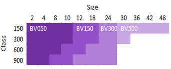
\*Size based on standard valve flange size \*Capacity based on standard BV capacity @ 1.5x ANSI psi
