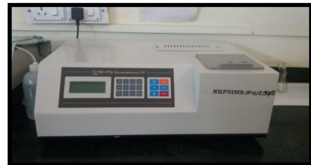
Figure 3: Calcium release is evaluated by Calcium Reagent Kit and measured by uv-vis Spectrophotometer.
