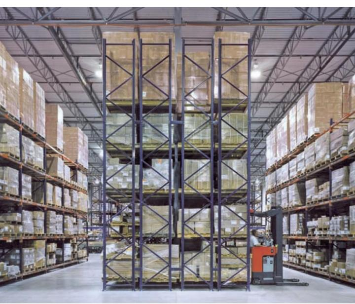
Double deep racking is created by placing 2 double sided runs together.
