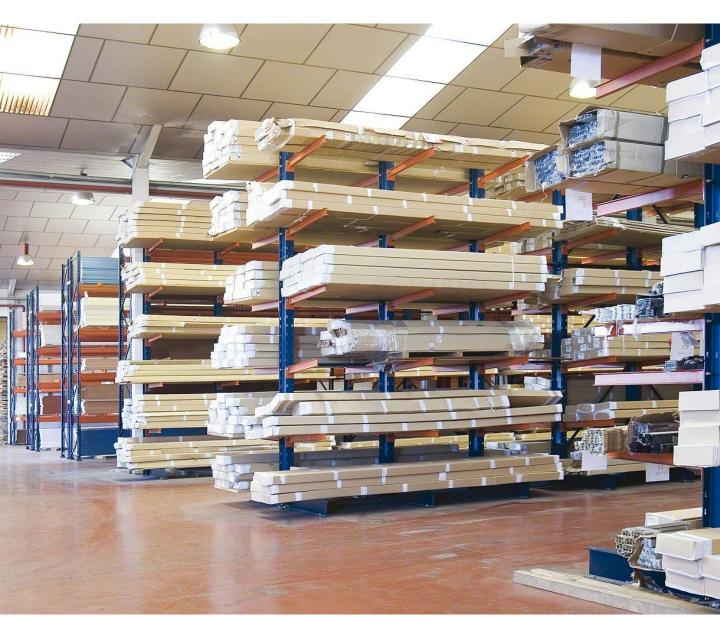
It is specifically designed to store long loads such as beams, profiles, pipes and timber. This rack enables loads to be handled by using lifting systems such as lift trucks, mobile cranes, stacker cranes, etc. These systems are chosen depending on the load to be stored (mainly weight and dimensions) or the height of the rack itself.
