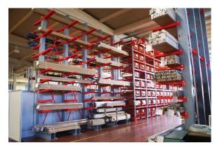
These racks are used to store rolls of carpet, wood, pipe, or any long mid-duty materials.
