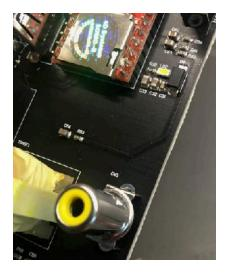
**AUX INPUT:** This RCA connector allows to input in the system an in-line sound thorugh the mixer of the sound board. This input is played by the board through the main output.
