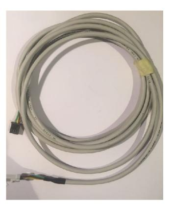
The DMX cable is used for bidirectional comunication from the driver board to the sound board. The sound board, which will be discussed later, is the one which interfaces with the ZA electronic set; this connection is done with a 6 rows<-> sound board cable; in case that the IP68 connector is used by switchpod relay board, the sound board can be connected to a ZA relay board.
