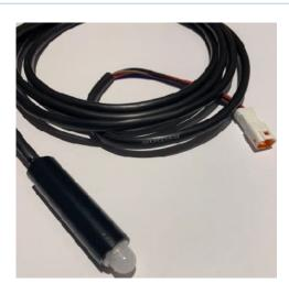
This cable is used to connect the (PIR) radar to the driver board. This cable, from one side end with the radar (PIR), keep in the appropriate support, to the other side instead, there is an IP68 connector. The lenght is 2 meters and can be fixed where you like. The suggestion is to fix it under the front bumper, near the center, between the fog lights for a better performance.
