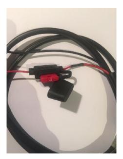
In order to avoid that more cables pass inside the car interior, it has been studied that the main power sits inside the engine bay. The drivers board has an integrated relay which interrupts power if the electronic set is switch off and of course it active when the dashboard is on. This also is done to avoid your battery drain during period of non-use.
