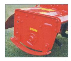
The machine can be center or offset mounted utilizing the moveable lower brackets.
