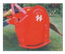
The machine is able to work up to 7" providing a fine tilth and an even finish.
