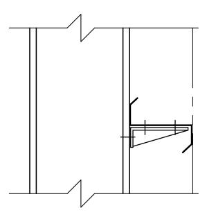
NOTES: BY-PASS CONDTION WITH FACTORY WELDED CLIP TO COLUMN
