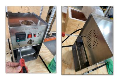
**4-6.** OPEN UP TOP PANEL AND SET OUT SO AS NOT TO PULL LOOSE ANY WIRES:
