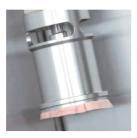
The vacuum gripper makes sure that the residual piece is kept as small as possible.
