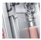
The patented vacuum gripper (optional) securely holds soft products such as boiled sausage, thereby ensuring increased production reliability.
