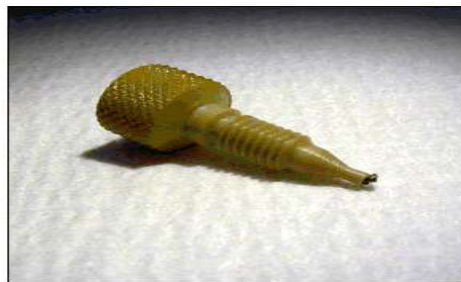
Tip shows foil matter accumulation
