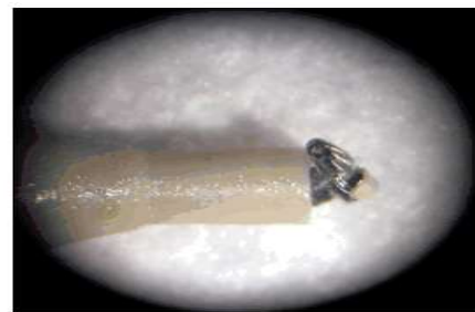
Tip filled with foil and adhesive (not cleanable)
