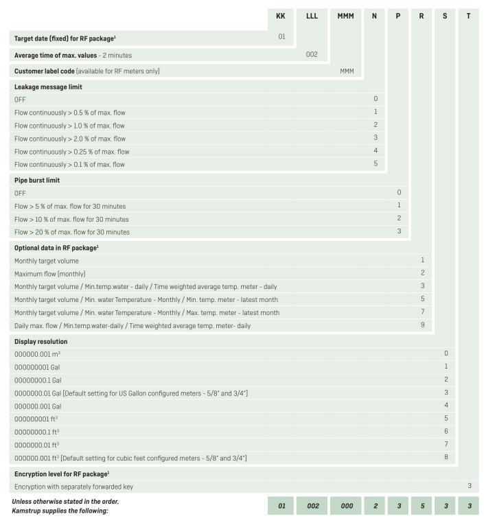
Note: 1) Configuration Codes KK, R and T affect only the RF version meter. Default values are used for EO meters, but serve no purpose.
