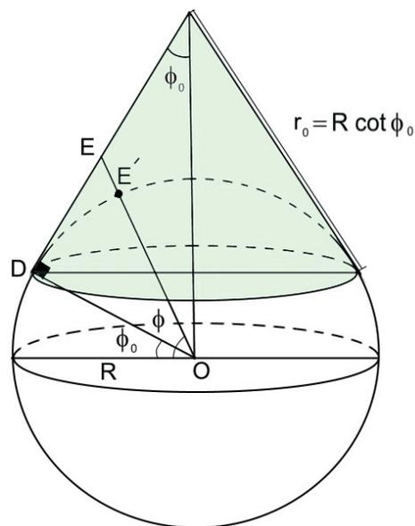
Figure 11: Geometry for the simple conic projection.
