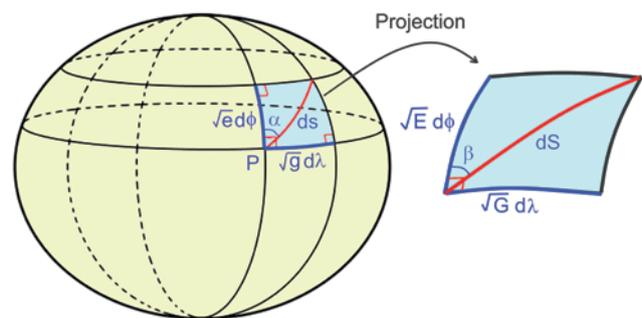
Figure 13: Geometry for differential parallelograms.
