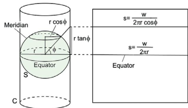
Figure 3: Geometry for the cylindrical projection.
