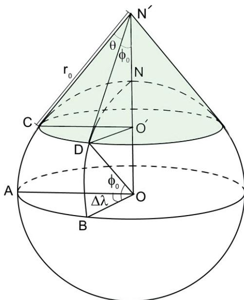
Figure 6: Geometry for angular convergence of the meridians.
