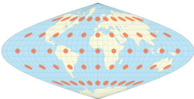
Figure 10: The sinusoidal equal-area projection.
