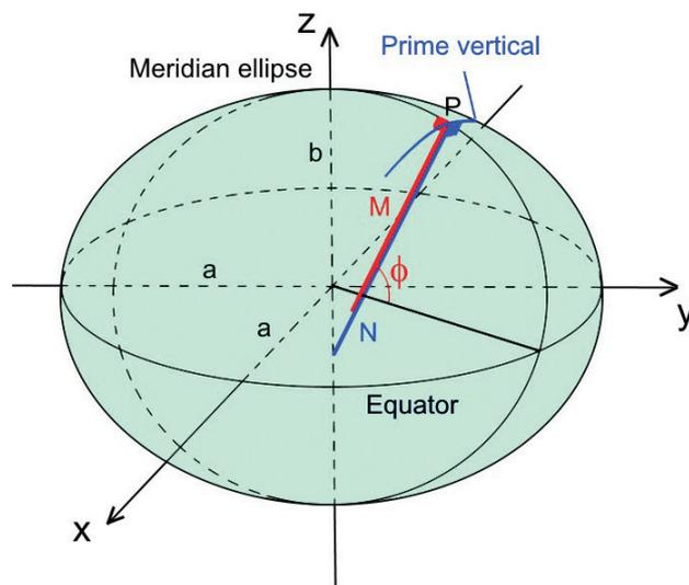
**Figure 2:** Geometry for the spheroidal model of the Earth,  $\frac{x^2}{a^2} + \frac{y^2}{a^2} + \frac{z^2}{b^2} = 1$ .
